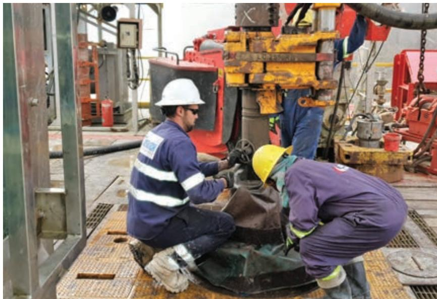
Fig. 4—The Non Stop Driller continuous-circulation system from Adrilltech has reduced connection times in harsh-environment projects.
