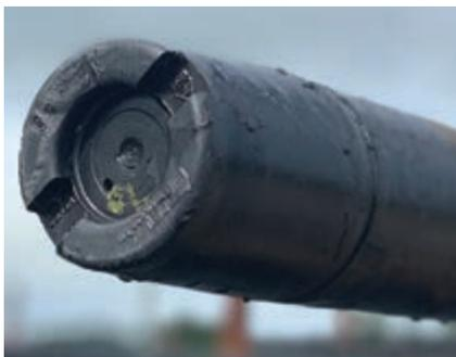
Fig. 3—NOV's Nano 25 rotary shoulder connection offers a cost-effective alternative to tubing.
